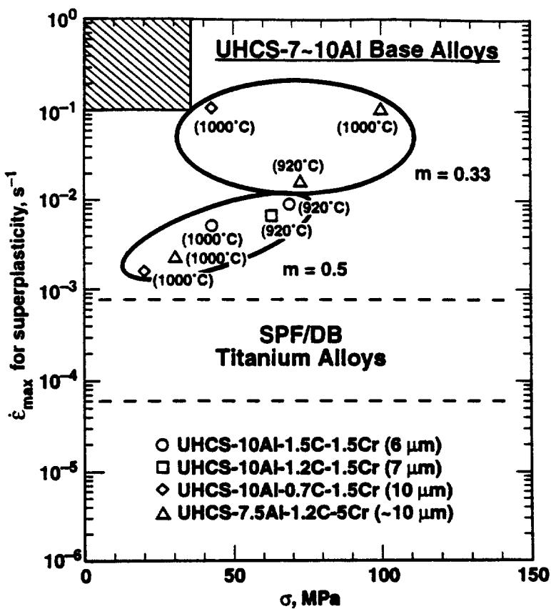
Figure 9. The maximum strain rate for superplastic flow, as a function of stress, for various UHCS-Al materials compared with the commercial goals set by the LLNL-industry consortium program (shaded area).
