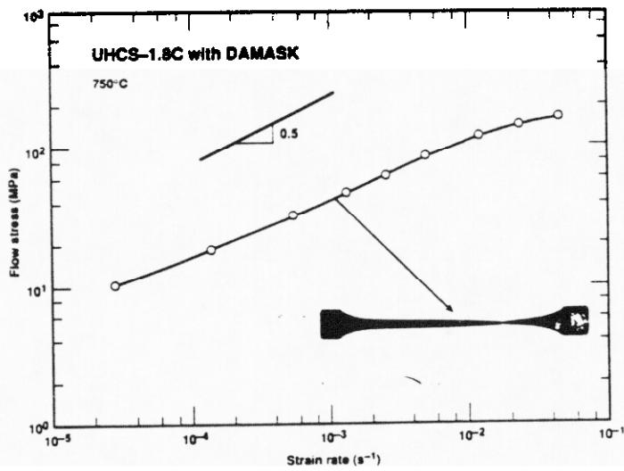
Figure 16. The flow stress-strain rate response of the UHCS material with visible damask at 750°C. The slope of the stress-strain rate curve shows a superplastic strain-rate sensitivity exponent of 0.43. The sample was tested at a strain-rate of 2% per minute to an elongation of 450%.
