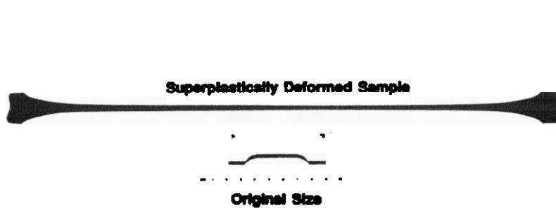
Figure 5. An example of superplastic behavior in an ultrahigh carbon steel containing about 1.8 percent C; an elongation of over 1,000 percent was achieved with no evidence of imminent failure.
