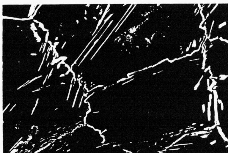
Figure 3. Micrograph of a modern ultrahigh carbon steel clearly showing a cementite network. The background structure is pearlite, i.e., alternating layers of essentially pure iron and iron carbide. (Magnification about 200 diameters.)
