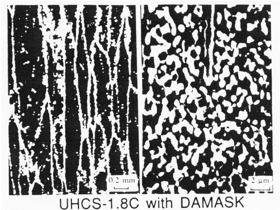
Figure 14. Photomicrographs of a UHCS-1.8 C material, processed by the Wadsworth-Sherby recipe. The photomicrograph on the left shows the proeutectoid carbide network with coarse dimensions of about 0.2 mm x 2 mm.
