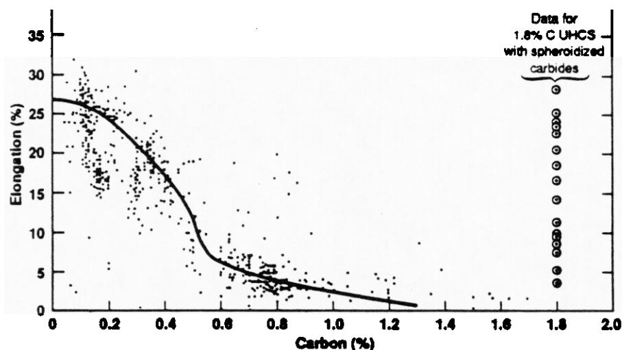
Figure 2. Historical data for the tensile elongation for steel at room temperature dramatically decreases as the carbon increases. (Reproduced from a book by the American metallurgist, Henry Howe, in 1891). Modern UHCSs can have far greater tensile elongations as shown by the data for a 1.8% C UHCS.
