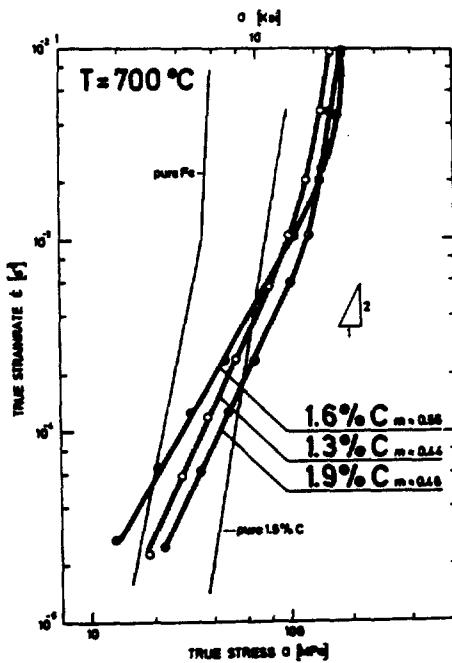
Figure 6. Comparison of the creep properties of UHCSs with pure iron and with a pure Fe - 1.6% C alloy.
