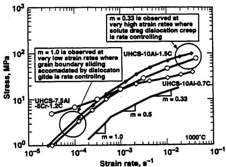
Figure 7. Quasi-superplasticity ( $m = 0.33$ ) and ideal grain-boundary sliding ( $m = 1.0$ ) are observed in UHCS-high aluminum alloys.
