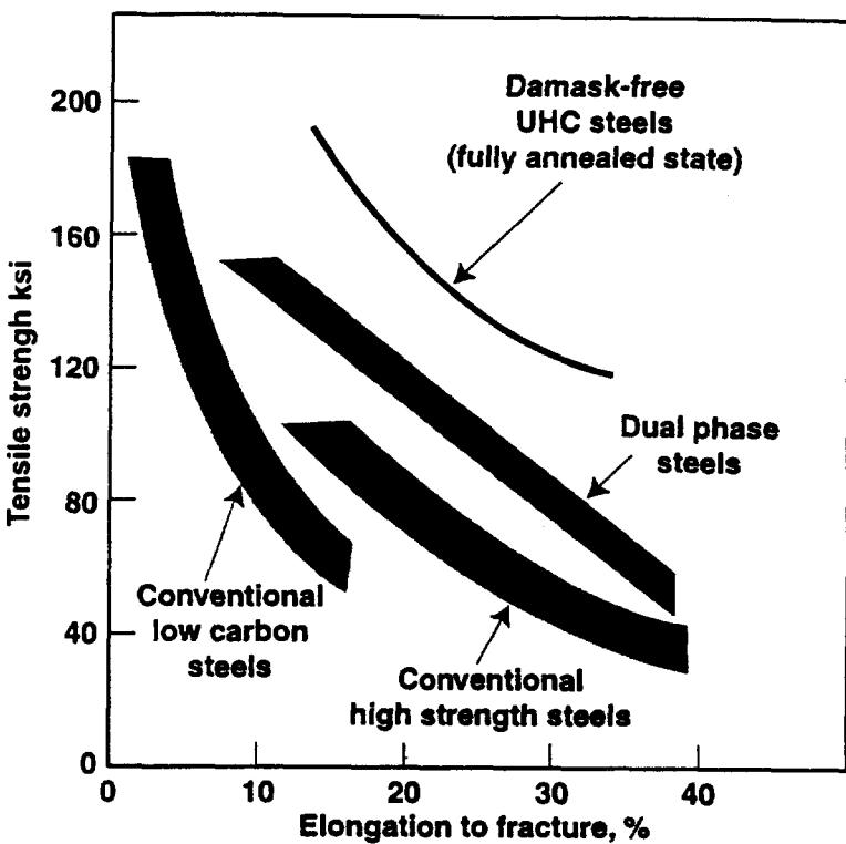
Figure 10. The considerable increase in strength of ultrahigh carbon steel sheet over conventional and advanced automotive steel sheet is illustrated when they are compared at an equivalent tensile ductility. The various strengths in the UHCS materials are achieved by different processing procedures and heat treatments ( $\text{ksi} \times 6.895 = \text{MPa}$ ).
