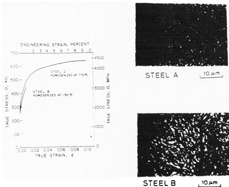
Figure 11. The influence of prior heat treatment on UHCS quenched from 770°C is shown in the above figure. On the graph, the compression stress-strain curves of a 1.3% C steel after two different prior heat treatments are shown with accompanying optical micrographs. The heat treatments involved, in one case heating to 770°C and quenching, and in the other case heating to 1150°C, cooling to 770°C, and then quenching.
