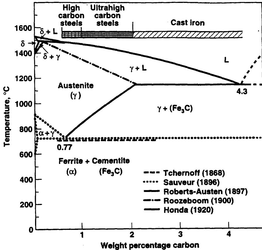
Figure 1. Historical description of the Fe-C phase diagram.
